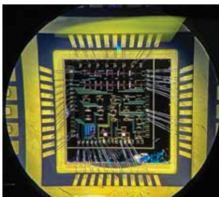
Electronic devices with gallium nitride transistors could be used in nuclear sensing equipment due to their high resistance to radiation.
