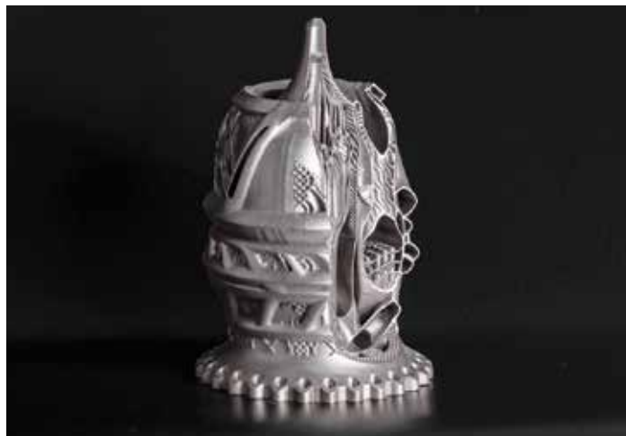
3D-printed combustion chamber highlights the advanced capabilities of metal additive manufacturing in aerospace, showcasing intricate and complex geometries that enhance engine performance and efficiency.
