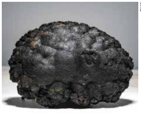
Polymetallic nodules have high concentrations of cobalt, manganese, and nickel.
