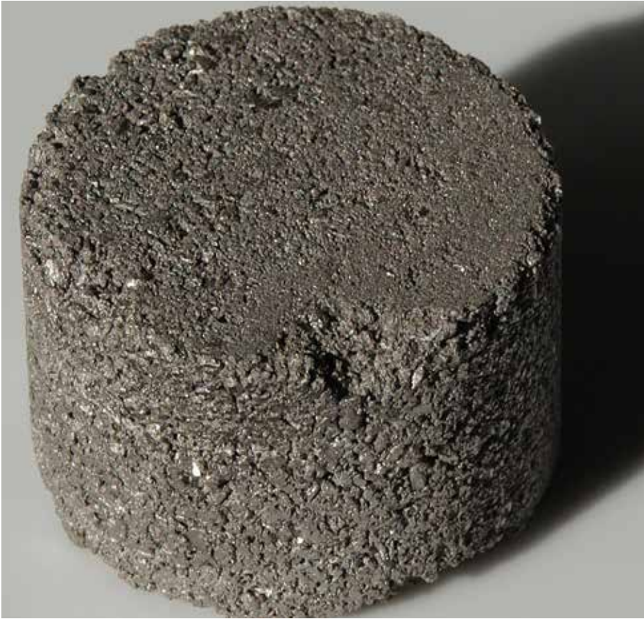
A puck of titanium sponge, the porous form of titanium created during the initial processing of the ilmenite or rutile, crucial for producing aerospace components and consumer goods.
