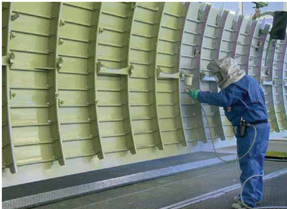
A technician applies a coating to aluminum-magnesium-scandium alloy – called AA5028 – developed by Aleris in collaboration with Airbus, highlighting the advancements in this critical mineral for aerospace and high-tech industries.
