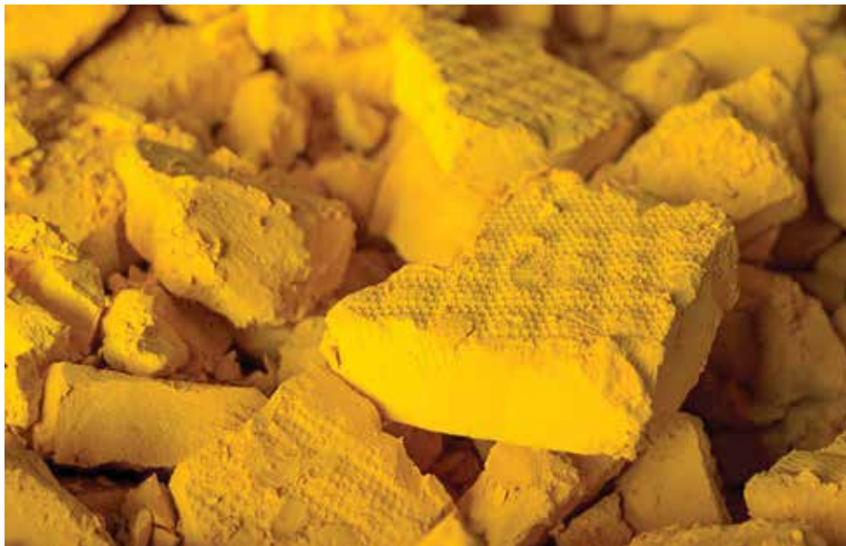
Uranium concentrate, called yellowcake, is used in the preparation of uranium fuel for reactors.
