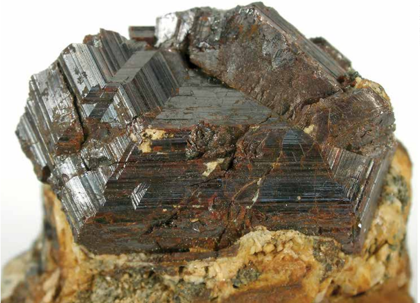
Rutile, a titanium-rich mineral, is essential for producing titanium dioxide, widely used in paints, plastics, and paper.
