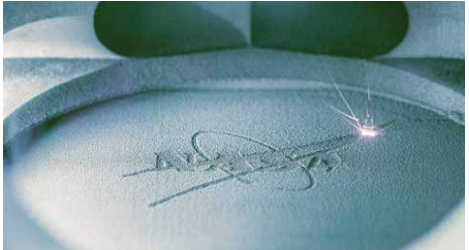
NASA's insignia is 3D printed with GRX-810, a superalloy designed for extreme durability.
